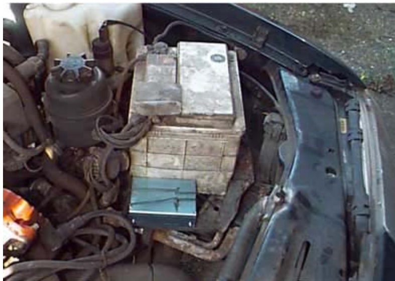
Figure 6. The data logger is located next to the car battery in perhaps the coolest area of the engine compartment. Car designers typically locate the battery in this area to prevent its electrolytes from boiling.
